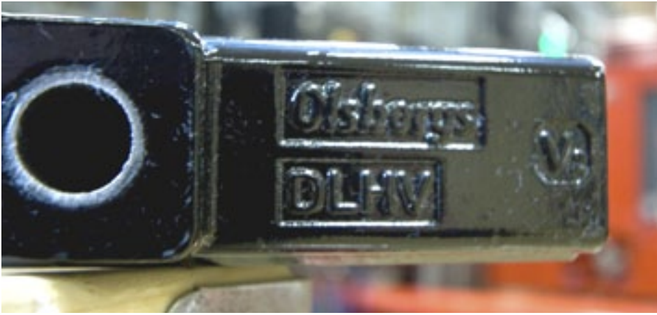
A cast valve body workpiece prior to processing with the Unimerco tool
