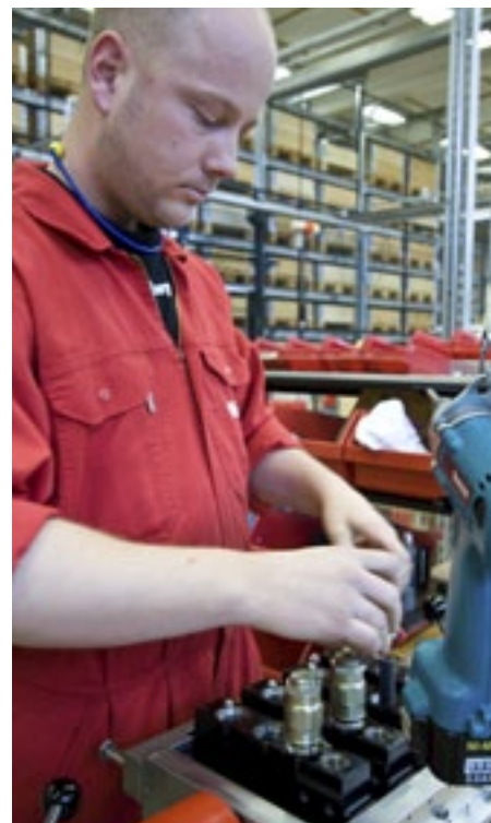
Rickard Ruther performing final assembly of the machined valve bodies that are then supplied, for instance, to crane manufacturers.
