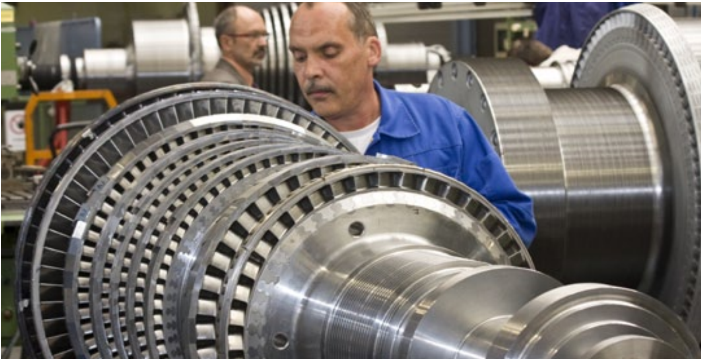
A turbine operating at a velocity of around 12,000 revolutions per minute exerts an enormous centrifugal force on the blades. The blades only make up one part of the roughly 3,000 components of a steam turbine – but they are also one of the most important for its correct functioning.
