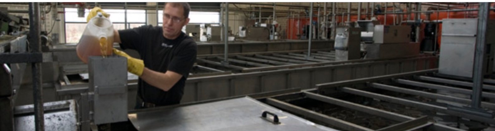
The coolant/lubricant system at Sunds
